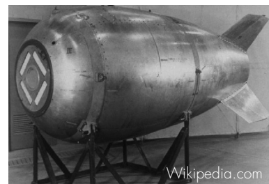
Mark IV bomb which used a 2,830 lb. steel casing.
